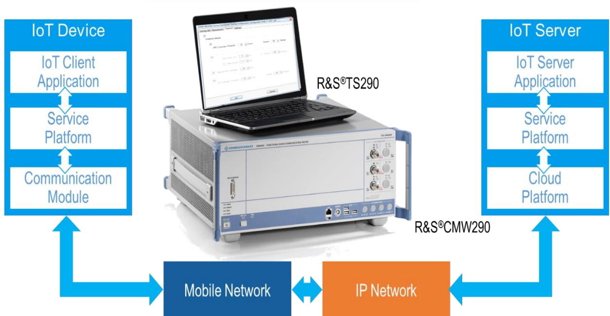
Figure : Using R&S®CMW290 for e2e application testing to check network-friendly behavior and performance in carrier acceptance testing in an R&S®TS290 test system
