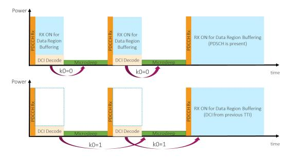
Figure 5-10 Same-slot (K0=0) vs. Cross-Slot (K0>0) Scheduling
