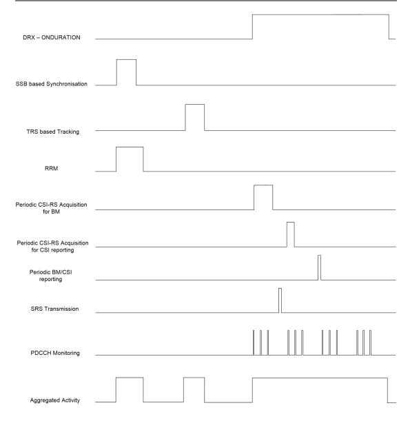
Figure 5-6 Processing Timeline including the Background activity.
