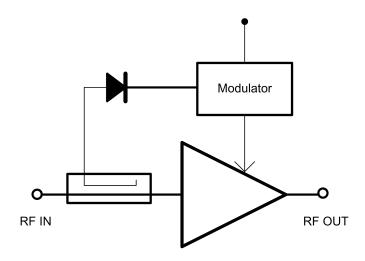
Figure 4-4 Envelope Tracking RF PA system
