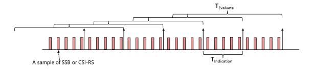
Figure 5-23: The UE procedures for RLM
