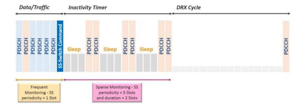
Figure 5-20: Example for SS-set group switching between sparse and dense PDCCH monitoring Rel-17 could consider the extensions to Rel-16 SS set group switching mechanism and the use of
