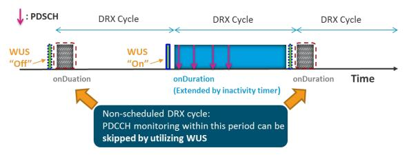
Figure 5-11 Wake UP Signal
