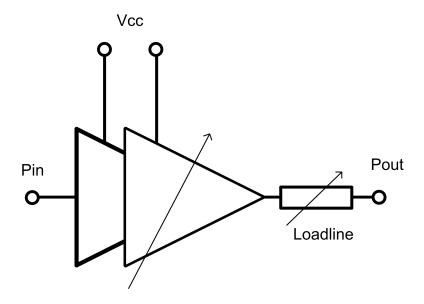
Figure 4-7 Topology of reconfigurable amplifier
