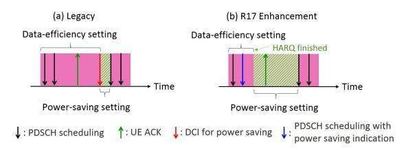
Figure 5-22: Power saving adaptation: (a) legacy and (b) R17 enhancement with pre-indication Initial analysis for both VoIP (FR1, 1 CC) and Real-Time-Video (FR2, 4CC) showed considerable gains as shown below, while minor latency degradation were seen specially in Video case
