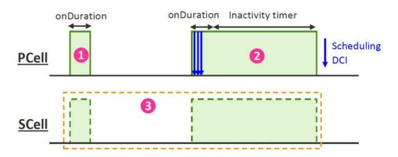
Figure 5-7 Release 16 power saving enhancements
