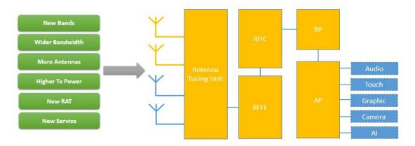
Figure 4-15G Device Block Diagram
