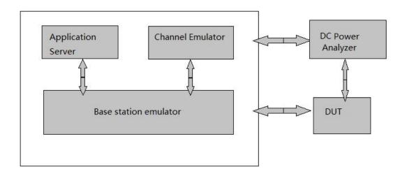
Figure 8-1 Common Test System Architecture
