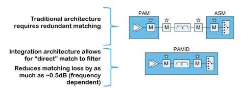
Integrated RF Front End as below is the best approach for 5G to save power consumption
