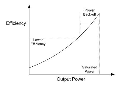
Figure 4-3 Typical relationship between efficiency and output power
