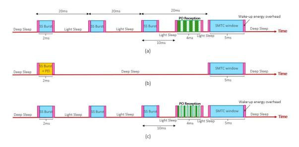
Figure 5-16: UE processing timelines: (a) Rel-15/16, (b) paging early indication, (c) UE grouping UE Group PEI (GPEI)
