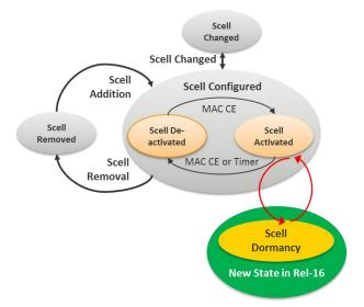
Figure 5-8 SCell State diagram for Rel-16
