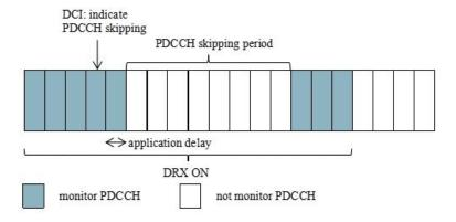
Figure 5-21: PDCCH skipping mechanism
