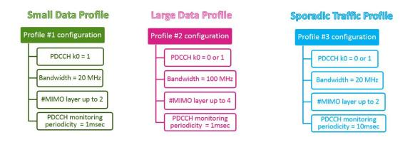
Figure 5-5 Examples of power profiles for different traffic characteristics
