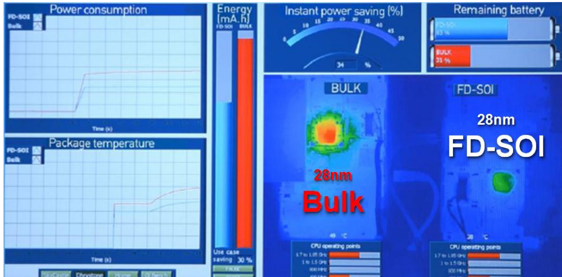
Figure 8-547 cellular microprocessors power saving FD-SOI versus bulk, STM
