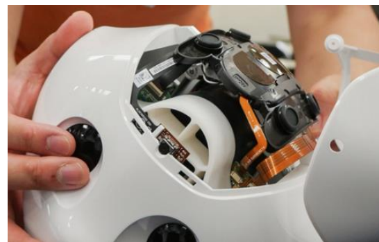
Figure 12: Microphone array and top camera in Pepper robot [Source: http://techon.nikkeibp.co.jp/article/COLUMN/20150623/424503/?P=2 ]
