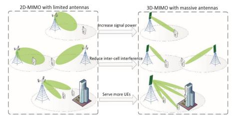
Figure 2-1 Technical principles of Massive MIMO
