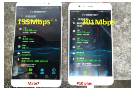
Figure 2: 4x4 MIMO terminal and common 4G terminal experience contrast
