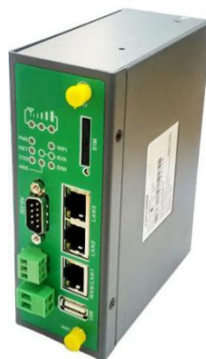
Figure 1-9. The shape diagram of an industrial intelligent gateway device
