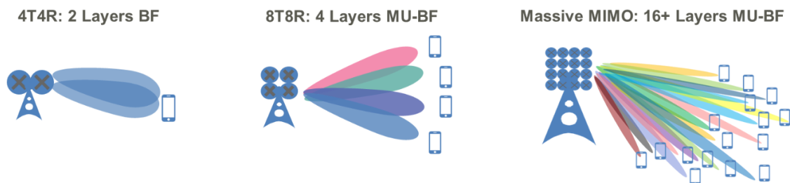
Figure 178 TDD Massive MIMO Comparison with TDD 4T4R/8T8R
