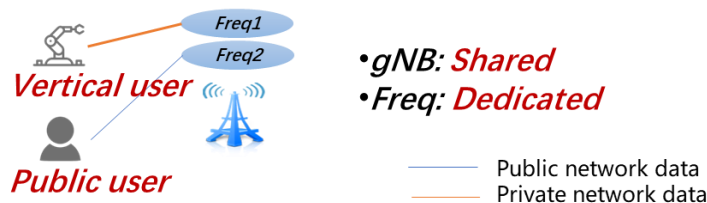
Figure 2-1 M-ENS architecture: The enterprise network reuses public network radio resources and occupies some frequencies
