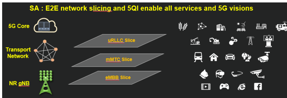
Figure 8.2 SA Provides End to end Network Slicing and 5QI for Better QoS Guarantee
