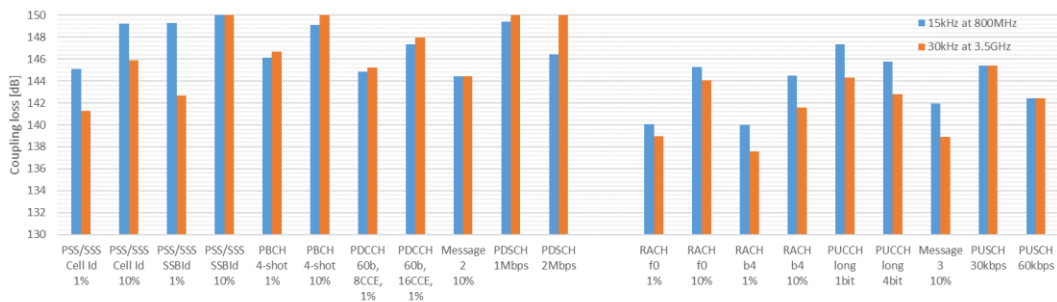
Figure 5-3 Preliminary results of maximum coupling loss for 15kHz numerology at 800MHz and 30kHz numerology at 3500MHz.
