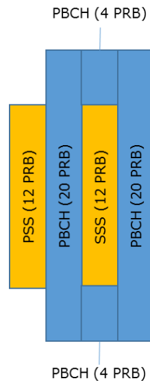
Figure 6-5 Illustration of SS/PBCH block mapping
