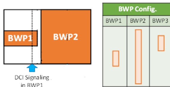
Figure 6-3 Illustration of DCI-based active BWP switching
