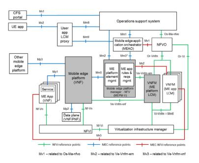
NOTE 1: It is assumed that the Mobile Edge Platform VNF, the MEPM-V and VNFM (ME platform LCM) will be deployed as a single package as per the ensemble concept in 3GPP TR 32.842 [i.8], or that the VNFM is a Generic VNFM as per ETSI GS NFV-IFA 009 [i.9] and the Mobile Edge Platform VNF and the MEPM-V are provided by a single vendor.
