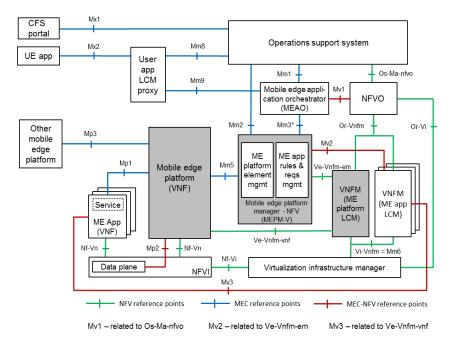
In This reference architecture, the management and orchestration of MEC is divided into two parts
