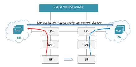
The 5G Core Network may expose network information and capabilities to an Edge Computing Application Function. Depending on the operator deployment, certain Application Functions can be allowed to interact directly with the Control Plane Network Functions with
