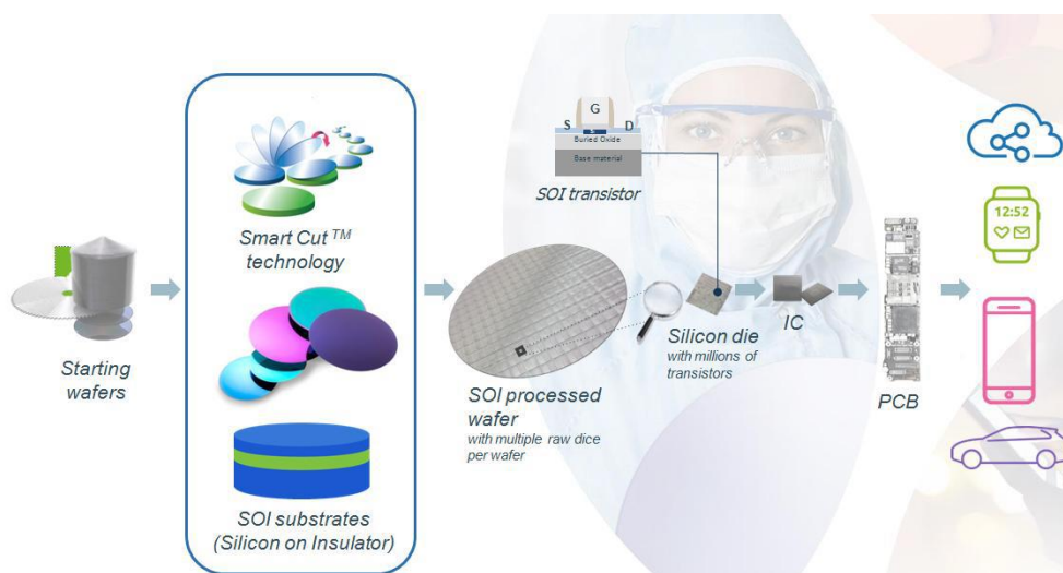
Figure 8-1 Engineering substrate in the supply chain, Soitec
