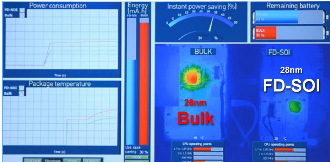
Figure 8-58 cellular microprocessors power saving FD-SOI versus bulk, STM
