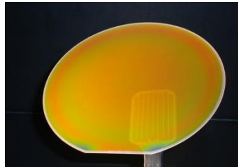
Figure 8-13 Bonded Silicon on Sapphire, Soitec
