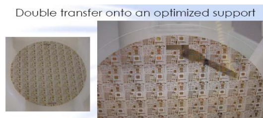
Figure 8-14 SOI devices transferred onto 200mm fused silica wafer, Soitec
