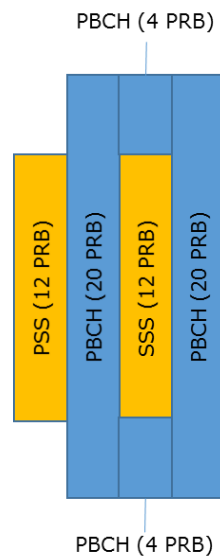
Figure 5-2 Illustration of SS/PBCH block mapping
