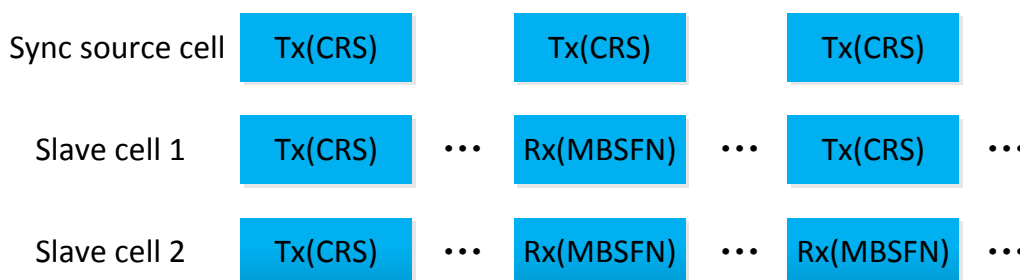
Figure.5 Tracking based on MBSFN subframes
