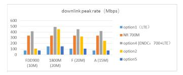
Figure 3-10 The theoretical analysis of the downlink peak rate of NR 700M and Option 1/2/4/5
