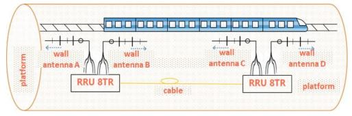
Figure 3-30 The new tunnel wall antenna scheme deployed in subway scenarios
