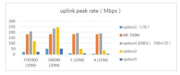
Figure 3-9 The theoretical analysis of the uplink peak rate of NR 700M and Option 1/2/4/5
