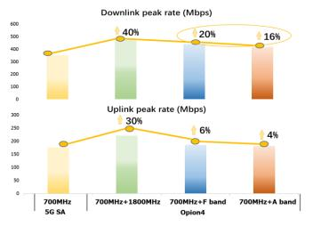
Figure 3-8 The theoretical analysis of the uplink and downlink peak rate of Option 4
