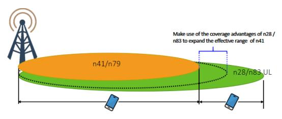
Figure 3-1 The SUL architecture
