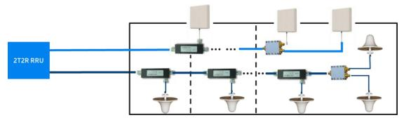
Figure 3-24 The DAS+Panel Antenna with multi-channel joint transceiver technology
