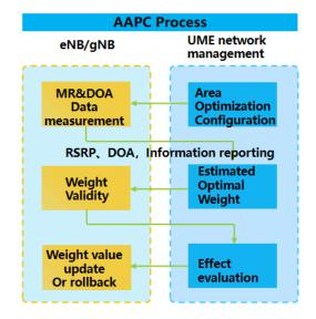
Figure 4-15 Automatic Antenna Pattern Control
