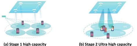
Figure 3-20 SuperMIMO improves cell capacity in high value scenarios
