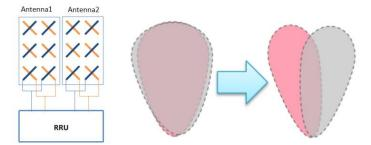
Figure 3-34 The beam becomes narrow after the beamforming and 2 SSB works simultaneously
