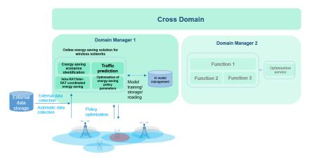
Figure 4-28 Architecture of the online energy-saving solution for wireless networks
