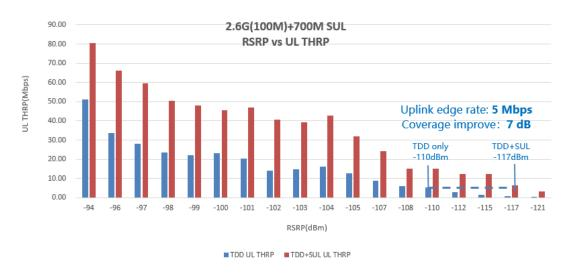
Figure 3-5 2.6G+700M SUL test results
