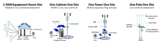
Figure 4-33 The transformation of construction mode
