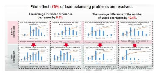
Figure 4-14 Pilot result of load balance with intelligent multiple parameter optimization
