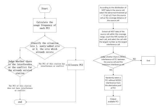
Figure 4-24 The PCI Interference/Conflict Detection Algorithm Based on the Distance and MDT
