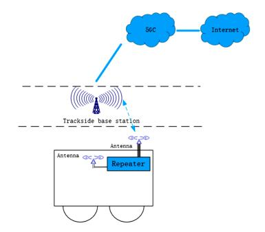
Figure 3-29 The repeater solution network architecture diagram
