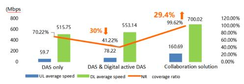
Figure 3-17 Collaboration solution has better performance in field drive test
