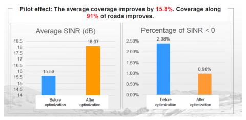
Figure 4-8 Pilot result of the NR network coverage before & after the optimization
