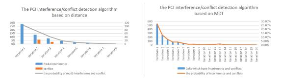
Figure 4-25 The Validation Results of PCI Interference/Conflict Detection Algorithm Based on Distance and MDT
