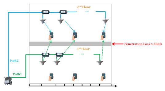
Figure 3-22 The cross-floor MIMO based on single-path DAS
