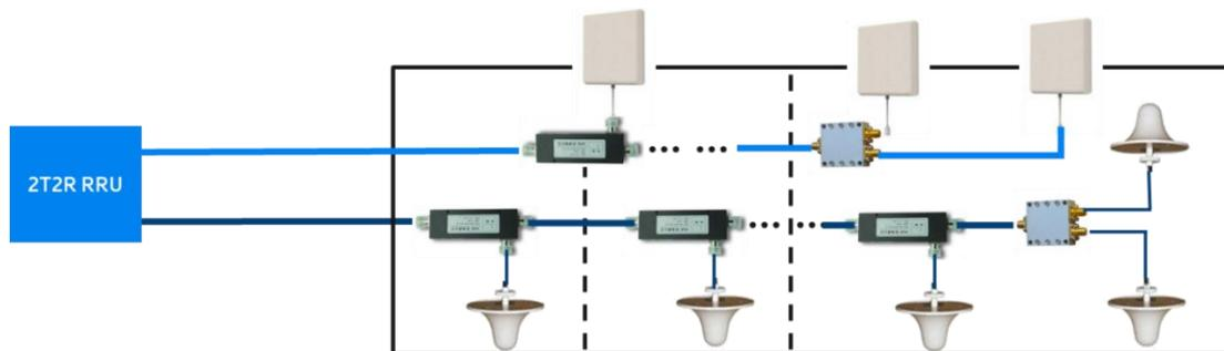
**Figure 3-24 The DAS+Panel Antenna with multi-channel joint transceiver technology**
