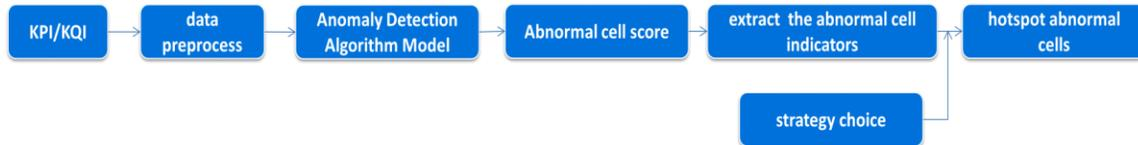
**Figure 4-16 The Architecture of the Anomaly Detection Application**
