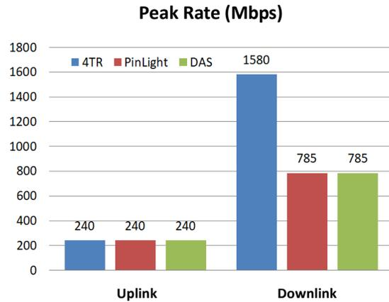
Figure 3-13 Comparison of peak rates of 4TR active DAS, N-point Joint Networking and dual-path passive DAS
