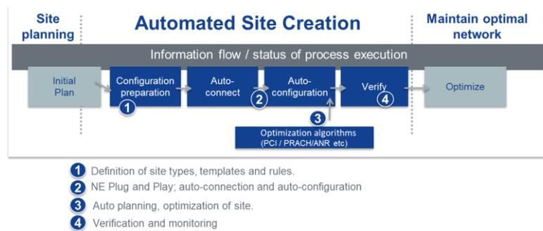
**Figure 4-3 The diagram of ASC**
