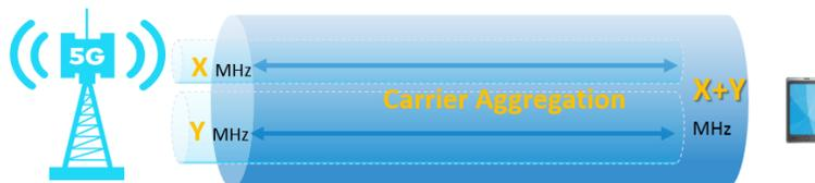
Figure 3-3 Carrier Aggregation
