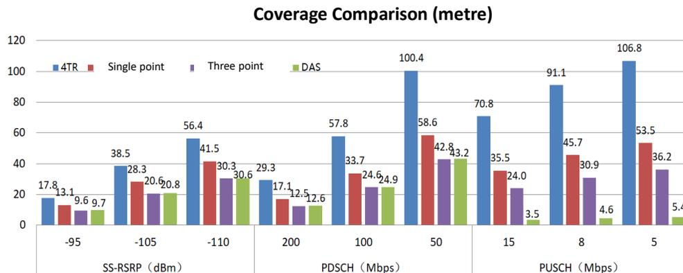
Figure 3-15 Comparison of coverage of 4TR active DAS, N-point Joint Networking and dual-path passive DAS
