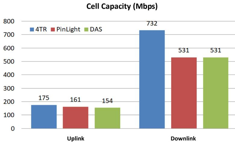
Figure 3-14 Comparison of cell capacity of 4TR active DAS, N-point Joint Networking and dual-path passive DAS
