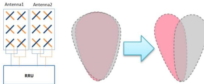
**Figure 3-34 The beam becomes narrow after the beamforming and 2 SSB works simultaneously**
