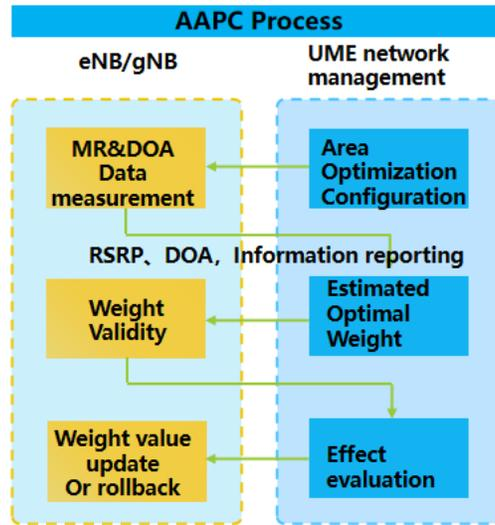
Figure 4-15 Automatic Antenna Pattern Control
