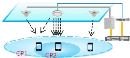
Figure 3-16 Overlay deployment for capacity
