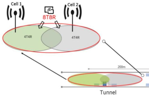
Figure 3-31 Multi-sector per radio 8TR splitting into two 4TR
