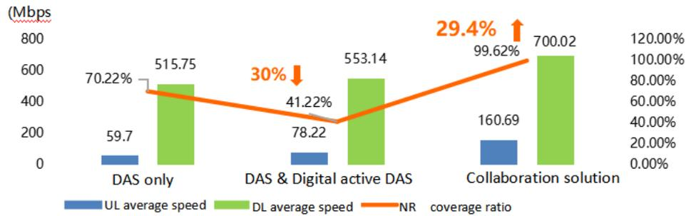
**Figure 3-17 Collaboration solution has better performance in field drive test**
