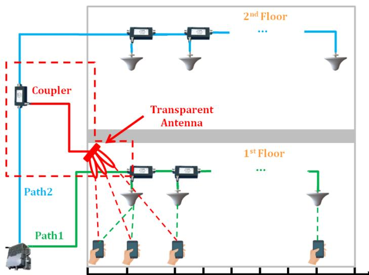
Figure 3-23 The local area MIMO under single-path DAS
