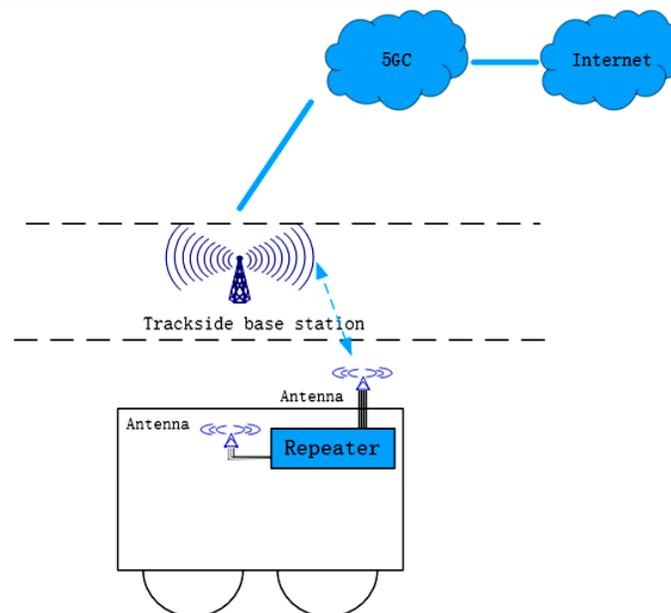
**Figure 3-29 The repeater solution network architecture diagram**
