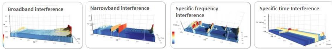
Figure 4-19 The visual interference diagram
