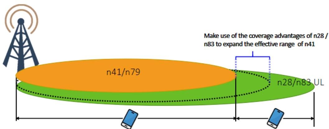
**Figure 3-1 The SUL architecture**
