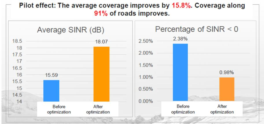
**Figure 4-8 Pilot result of the NR network coverage before & after the optimization**
