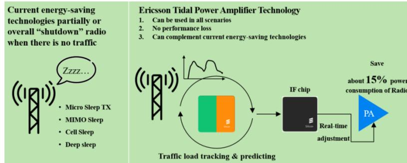
**Figure 4-32 Tidal Power Amplifier Technology**
