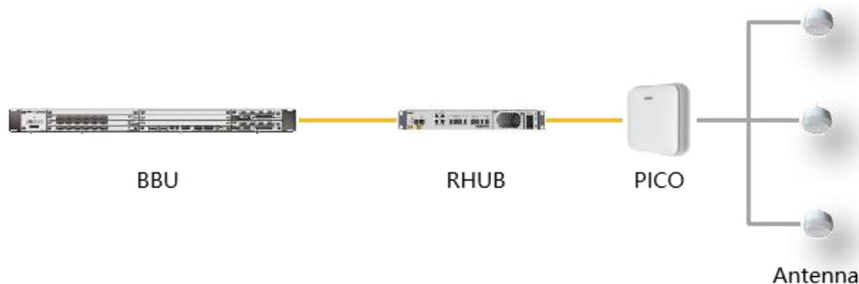
**Figure 3-11 The new joint networking solution**
