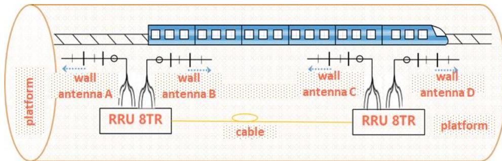
Figure 3-30 The new tunnel wall antenna scheme deployed in subway scenarios
