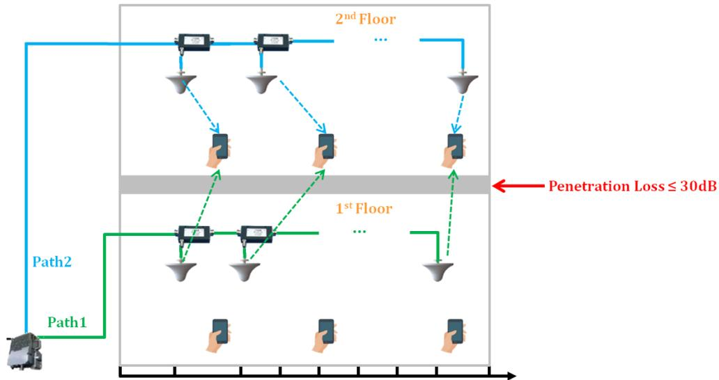
Figure 3-22 The cross-floor MIMO based on single-path DAS
