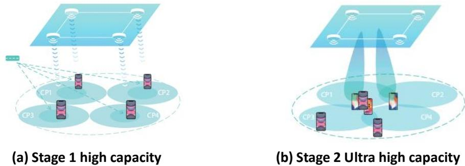
Figure 3-20 SuperMIMO improves cell capacity in high value scenarios
