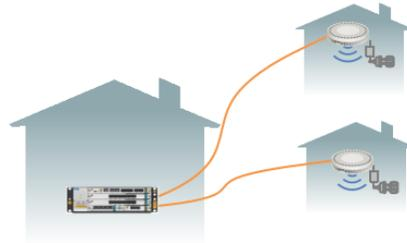
**Figure 3-19 Simplified Digital Active DAS supporting direct connection between BBU and Pico RRU**
