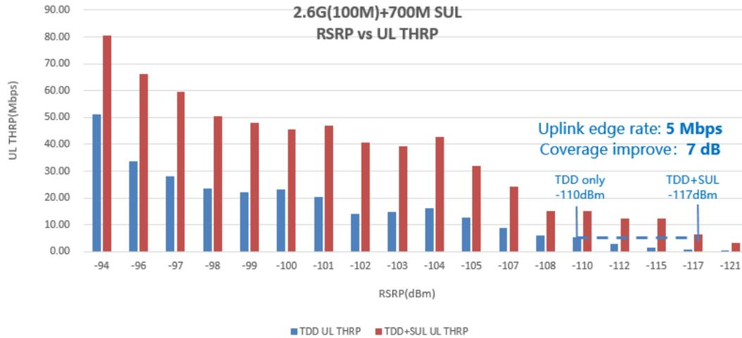
Figure 3-5 2.6G+700M SUL test results
